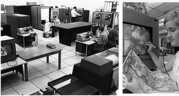
Fig. 8. Purdue University's LARSYS computer system, circa 1971 (left). The world's first digital image display, developed by IBM for LARS, can be seen in the center-left. Using an electronic interface pen, analyst Kay Hunt uses interactive pen technology to locate training pixels on the digital display (right) (L. Biehl, LARS).
