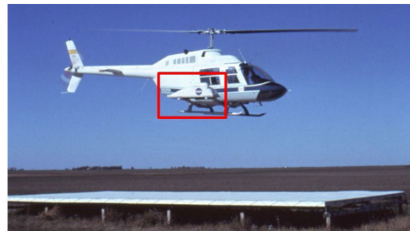
Fig. 25. Field spectrometer system (FSS) is in the pod on the side of the NASA helicopter (inside the red box) [73].
