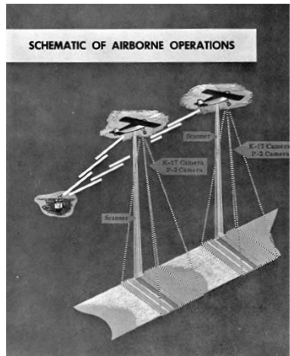
Fig. 1. Flight configuration of the two-aircraft (L-20) each containing a prototype WRL multispectral scanner system. Each pilot used the same visual ground object to maintain the same flight path. Combining the various imaging systems made coregistering of the data problematic [4].
