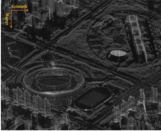
Fig. 4. Mean-intensity map from 26 SAR images of an urban area over Shenzhen (Size: 1376 \times 3826 in the range-azimuth direction).
