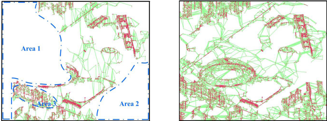
Fig. 8. Distribution of the constructed SRN (left) and AntRN (right). Area 1, Area 2, and Area 3 are the urban built areas that are not covered by the SRN. For both the SRN and the AntRN, the SPS arcs are marked with bright green lines and the SPSs are marked with red solid dots.
