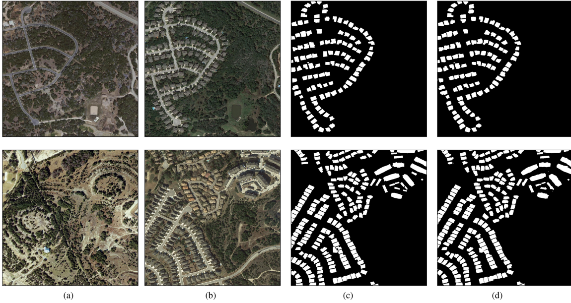
Fig. 12. 1024 \times 1024 pixel output visualization for LEVIR test images. (a) Image 1. (b) Image 2. (c) Ground truth. (d) Our Output.
