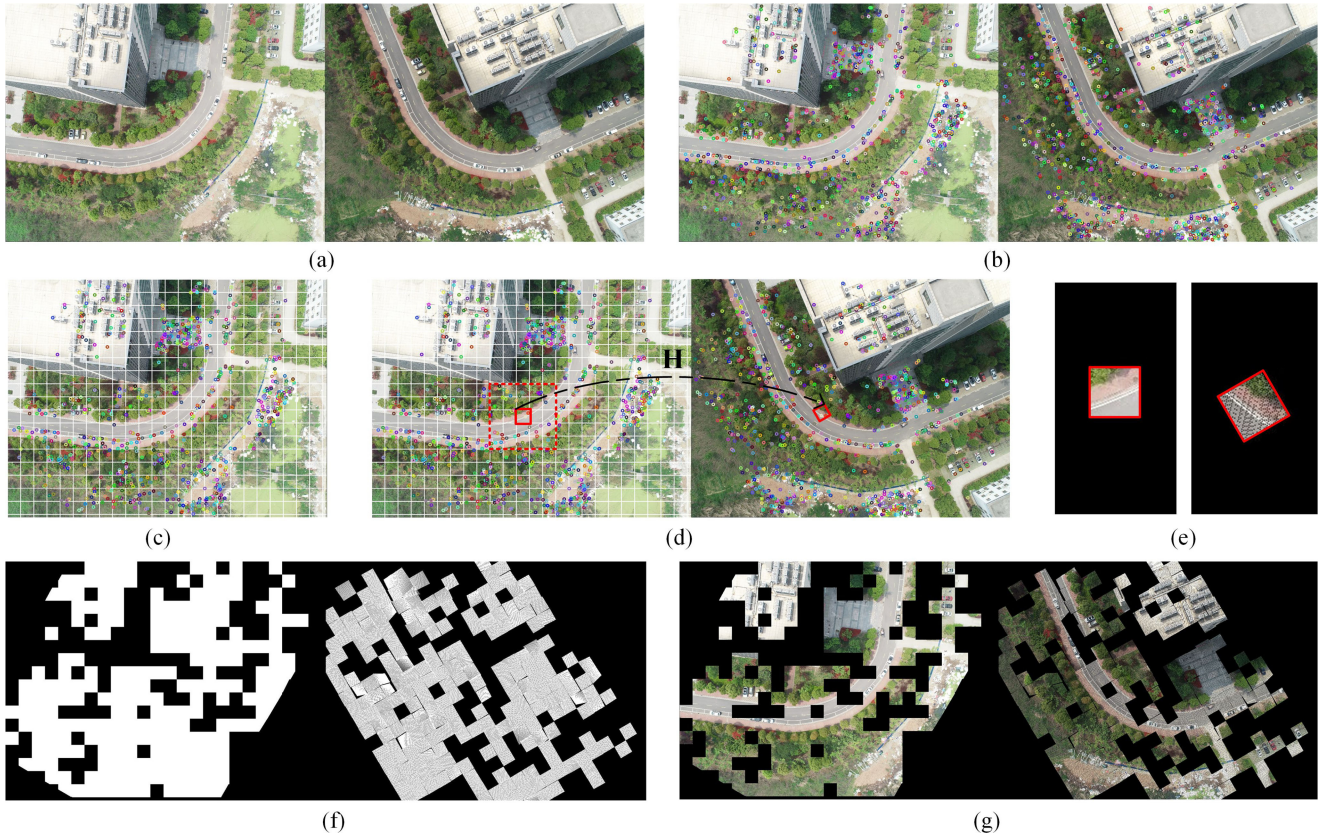
Fig. 3. Calculation process of the homography matching regions. (a) Original image pair. (b) Sparse matching points of two images. (c) Grid division of the first image. (d) For a valid grid that contains matching points, the local homography is calculated using the neighboring matching points. (e) Projection result of one grid. (f) Mask and (g) the final extracted matching regions.
