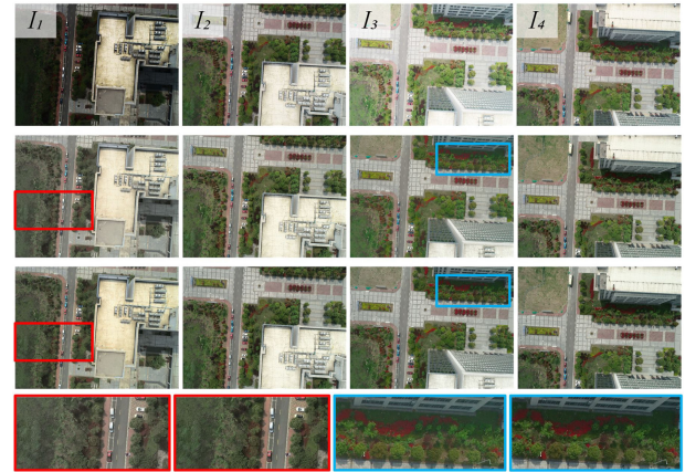
Fig. 4. (Row 1) Original images. (Rows 2 and 3) Correction results of the method using sparse matching points and our proposed method using homography matching pixels. (Row 4) Local enlarged details.
