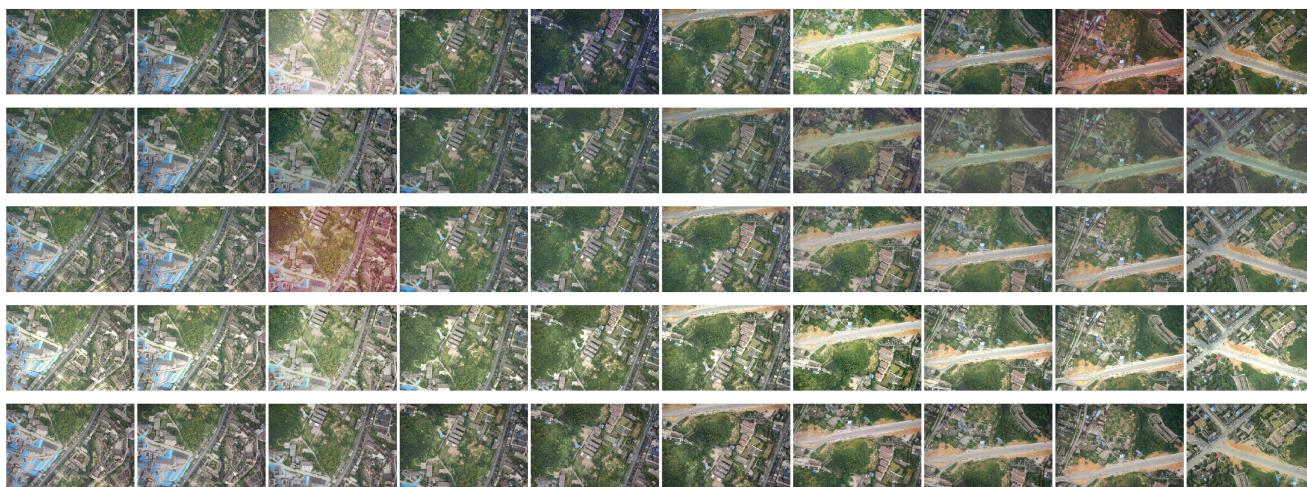
Fig. 9. Color correction results on YongZhou dataset. Limited by the space, only part of the images are displayed. (Row 1) Input images. (Rows 2–5) Results of Moulon et al. 's method [24], Park et al. 's method [4], Shen et al. 's method [25], and our proposed method.
