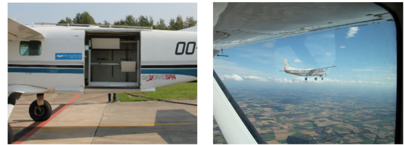
Fig. 1. MetaSensing BV's airborne L-band SAR system on-board one of the two CESNA Gran Caravan airplanes (left) and a picture of one airplane taken from the other while flying in the across-track (XT) configuration (right).
