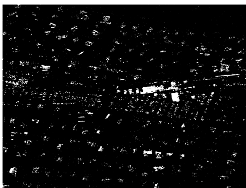
Fig. 4. Detection result obtained with the false alarm rate \alpha = 10^{-3} on the covariance matrices after correcting for the orientation angle with a bias, with the block-diagonal test statistic, at X-band.
