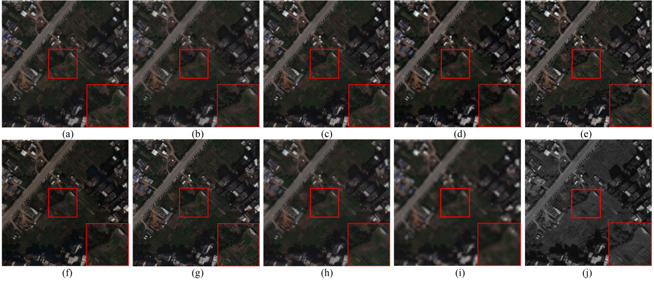
Fig. 6. Fused results by different methods on the WorldView-2 dataset. (a) GS. (b) MTF-GLP. (c) PRACS. (d) BFLP. (e) FSRIC. (f) PanColorGAN. (g) Fusion-Net. (h) Proposed. (i) MS. (j) PAN.
