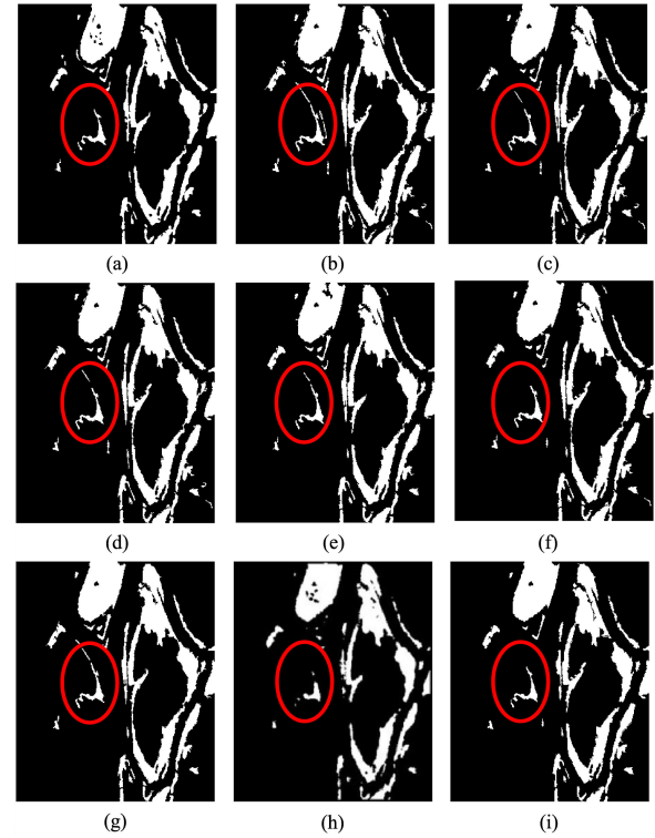
Fig. 14. Visualized results of different change detection methods on the Ottawa dataset. (a) Ground-truth image. (b) Result by PCAKM. (c) Result by NR-ELM. (d) Result by GaborPCANet. (e) Result by LR-CNN. (f) Result by MLFN. (g) Result by DBN. (h) Result by DCNet. (i) Result by the proposed GKSNet.
