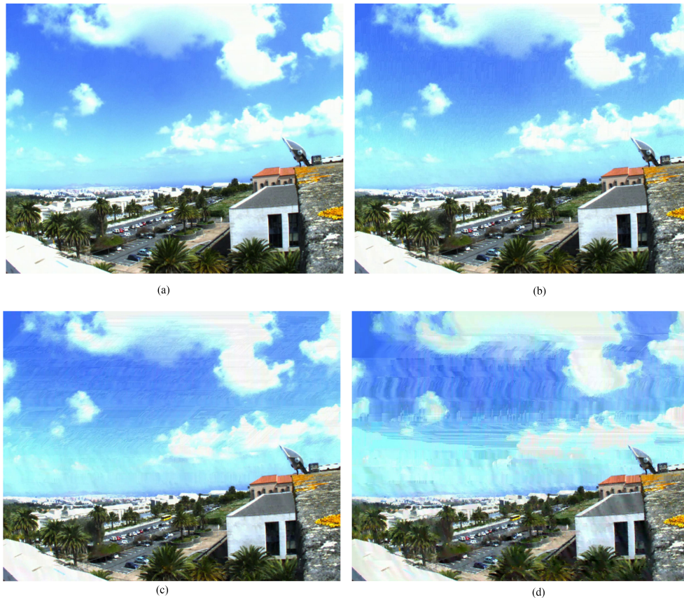
Fig. 13. Visual aspect of the decompressed frames from the Guagua video sequence when compressing it with different maximum errors values for the Y channel ( A_Y ) and for the Cb and Cr channels ( A_C ). (a) A_Y = 4 and A_C = 2 . (b) A_Y = 8 and A_C = 2 . (c) A_Y = 16 and A_C = 4 . (d) A_Y = 31 and A_C = 8 .
