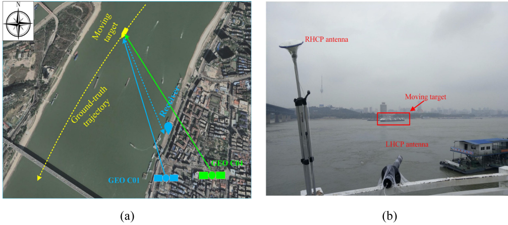
Fig. 5. Experimental scene. (a) Schematic diagram of the experimental GNSS-based radar acquisition geometry. (b) Experimental setup of the receiving system.
