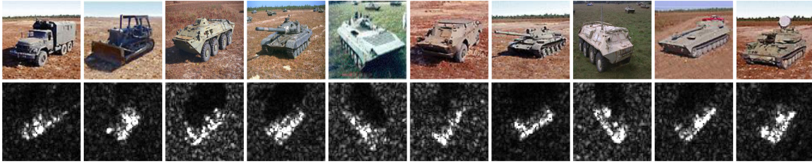
Fig. 7. Optical images (Top) and SAR images (Bottom) of MSTAR dataset. The class order is: ZIL131, D7, BTR70, T72, BMP2, BRDM2, T62, BTR60, 2S1, ZSU23/4.
