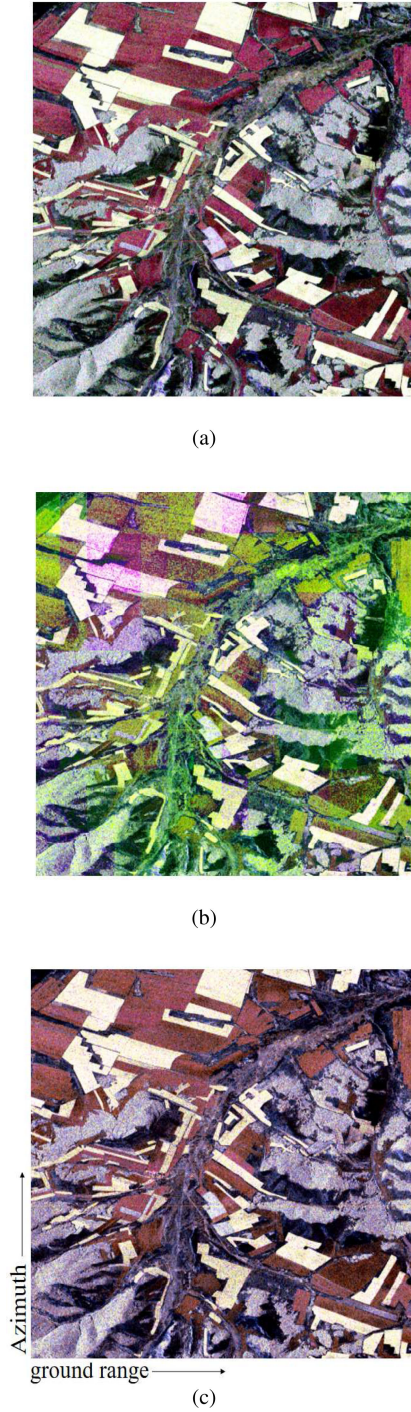
Fig. 20. Pauli-basis images of the reconstructed pseudo quad-pol data with different methods (GF-3). (a) Real quad-pol data. (b) QPRFCN. (c) CV-DBCNN. The red, green, and blue channels of the Pauli-basis image represent the double-bounce scattering, volume scattering, and single-bounce scattering, respectively.
