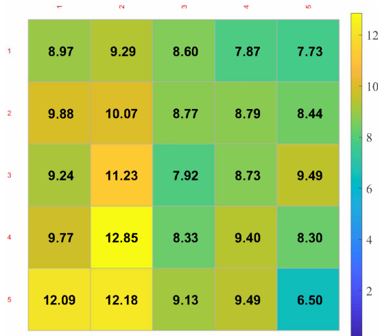
Fig. 8. Average value of cloud coverage error when the forecast time is 3 h.
