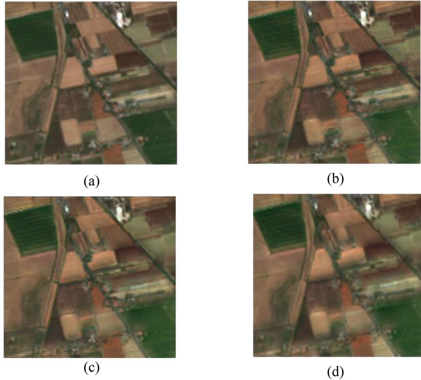
Fig. 10. RGB representations of the region of interest denoted as T : (a) Sentinel 2; (b) RSFIM-HP-hard; (c) RSFIM-HP-soft; and (d) SFIM-HP.
