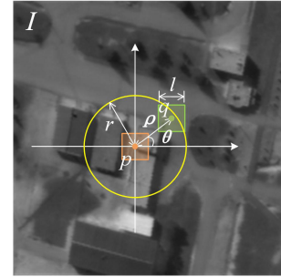
Fig. 2. Schematic of calculating the self-similarity of pixel p relative to pixel q . The red and green squares represent image patches centered on p and q , respectively.
