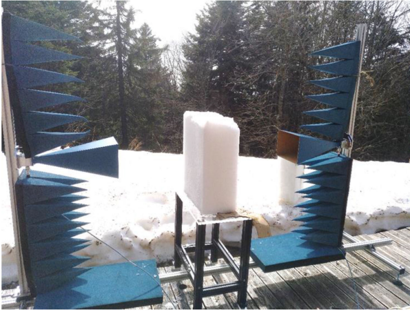
Fig. 3. Portable complex permittivity measurement bench.
