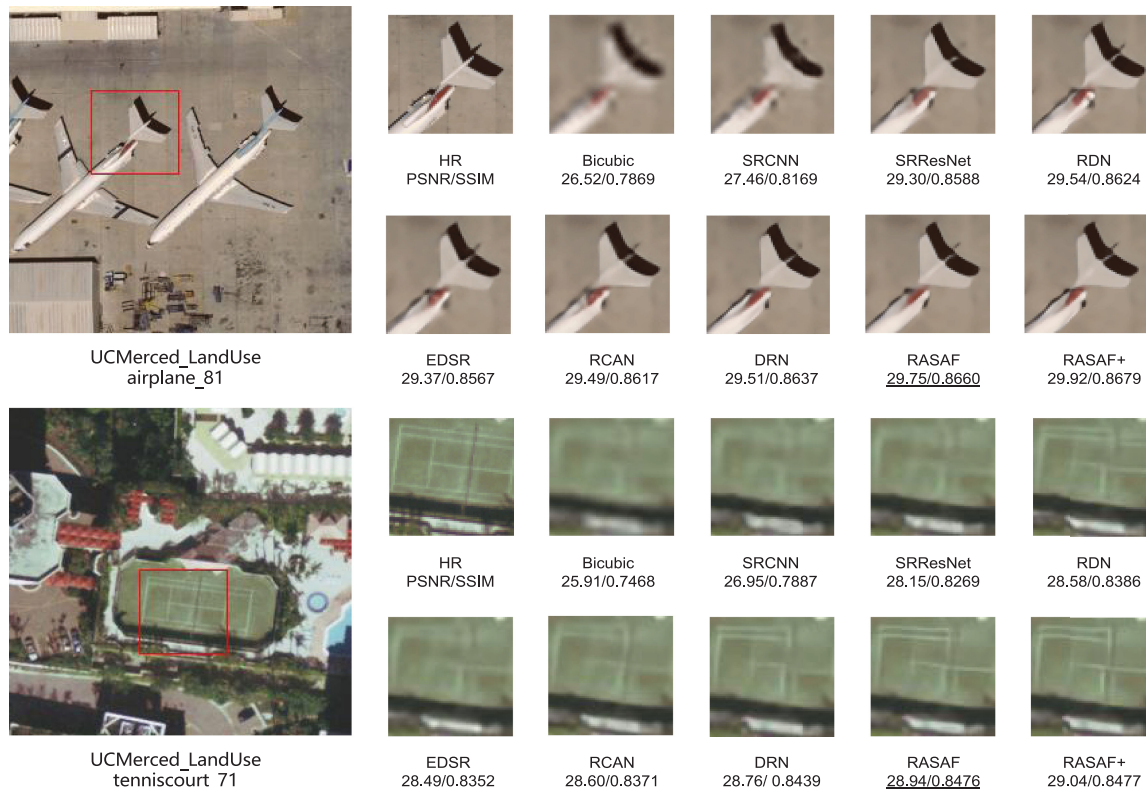
Fig. 5. Visualization comparison of various algorithms in the case of the UCMerced_LandUse with scale factor \times 4 .
