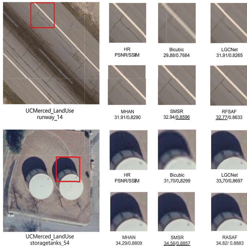
Fig. 7. Visualization comparison of remote sensing SISR algorithms in the case of the UCMerced_LandUse with scale factor \times 4 .
