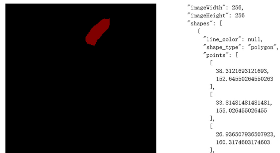
Fig. 7. Result of object segmentation. The edge is made up of points, and connecting these points together is the edge polygon of the target.
