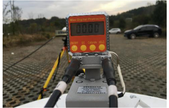
Fig. 19. Electronic level meter used in experiment.
