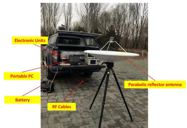
Fig. 2. Transponder for HY-2B altimeter in calibration.
