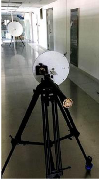
Fig. 12. Self-calibration of the transponder.
