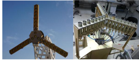
Fig. 11. FPASMR demonstrator. (Left) The L-band subsystem demonstrator. (Right) The X-band subsystem demonstrator.
