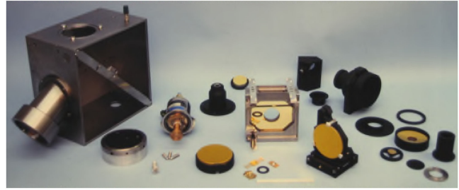
Fig. 12. Exploded view of the AIS instrument (Courtesy of NASA/JPL).
