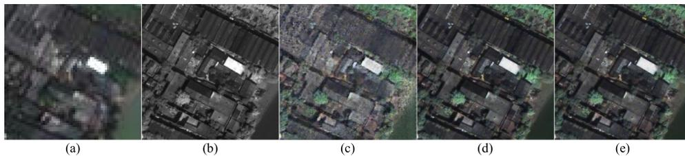
Fig. 15. Third group of fused image using different loss functions. (a) MS image. (b) PAN image. (c) LSGAN+PSNR. (d) LSGAN+L1. (e) LSGAN+L1+PSNR.
