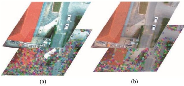
Fig. 7. Detection of key-points in a generated swath fragment. (a) Fragment of the RGB orthophoto mosaic. (b) Fragment of a hyperspectral swath.
