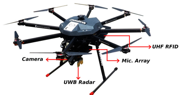
Fig. 1. Developed multisensory drone for disaster SAR mission [7], [8].
