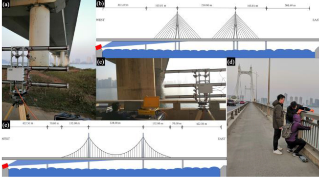
Fig. 3. (a) and (c) In situ measurement setup. (d) GPS receiver being installed on the bridge balustrade. (b) and (c) Sketches of the Yinpenling Bridge and Sanchaji Bridge, respectively.
