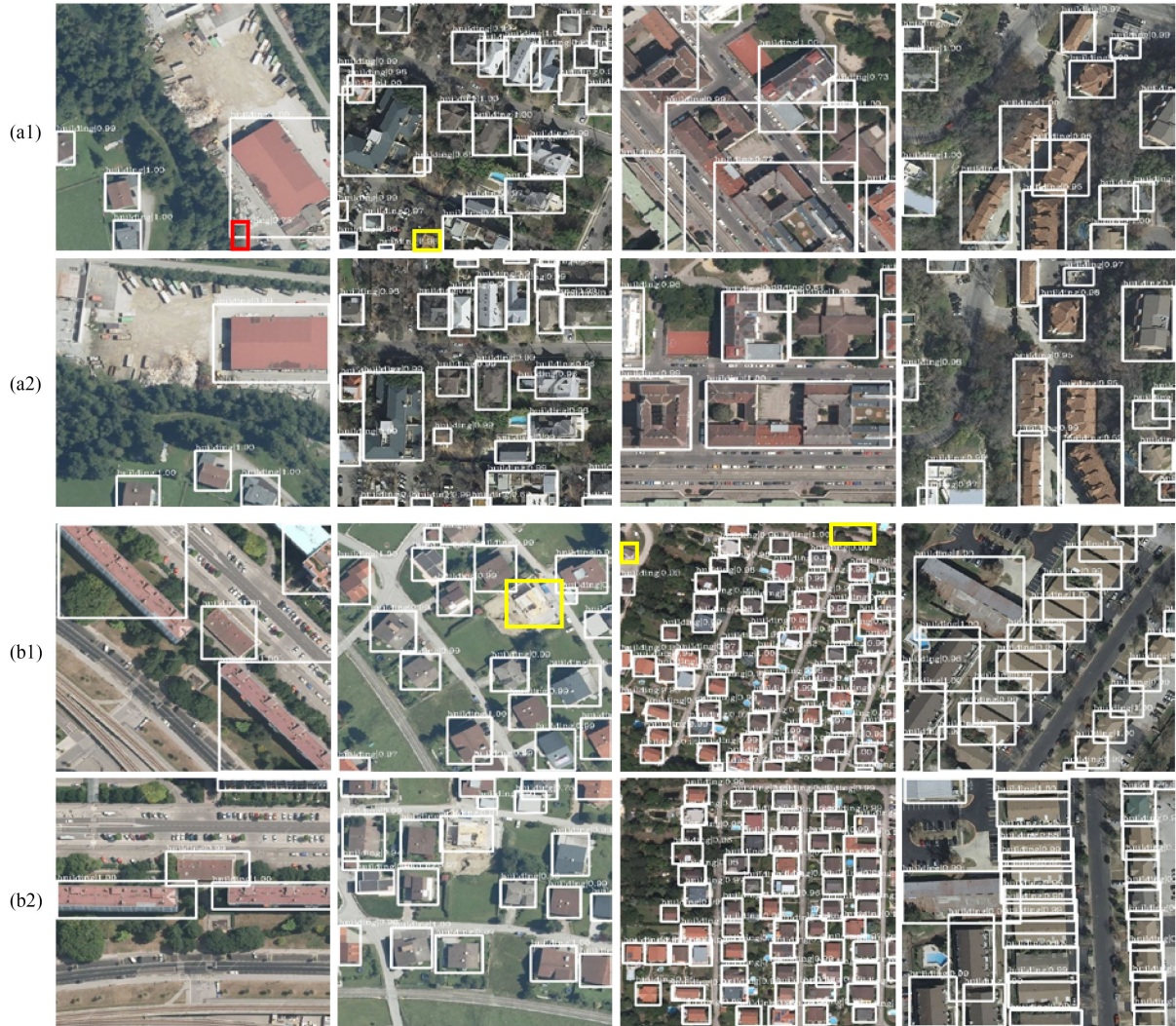
Fig. 8. Typical detection results of different scales, colors, and architectures. The results without TC are on rows (a1) and (b1), and the results with TC are on rows (a2) and (b2). The white bounding boxes are TPs, the yellow bounding boxes are FNs, and the red bounding boxes are FPs.
