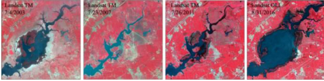
Fig. 4. Landsat images at different periods in the reservoir area. (The false-color composite images were created with RGB vs. NIR, Red, and Green bands).
