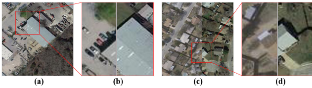
Fig. 1. Illustrations of (a), (b) geometric registration errors and (c), (d) spectral changes. We stitched the bitemporal images together and used the red boxes to highlight the pseudochanges. Zoom-in for an improved view. (b) and (d) are the local enlarged views of (a) and (c), respectively.
