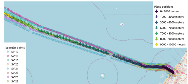
Fig. 3. Spread of the specular points received by an airplane taking off from the Dubai International Airport, depending on its height.
