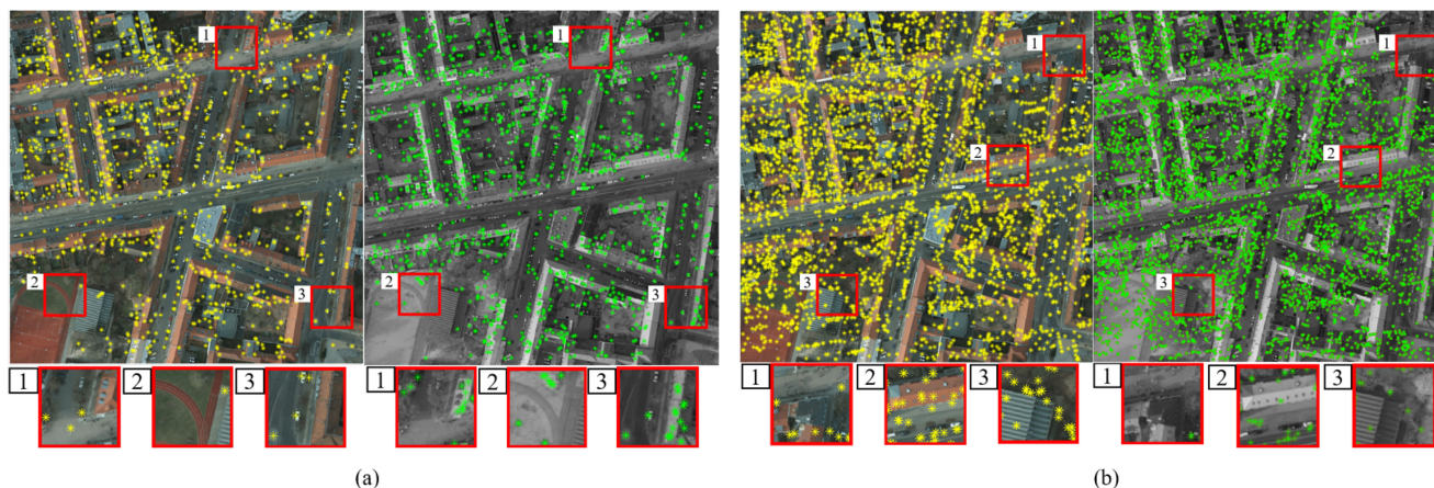
Fig. 1. (a) and (b) show the key points between optical (left) and NIR (right) urban remote sensing images, which are respectively detected by SIFT and SURF.
