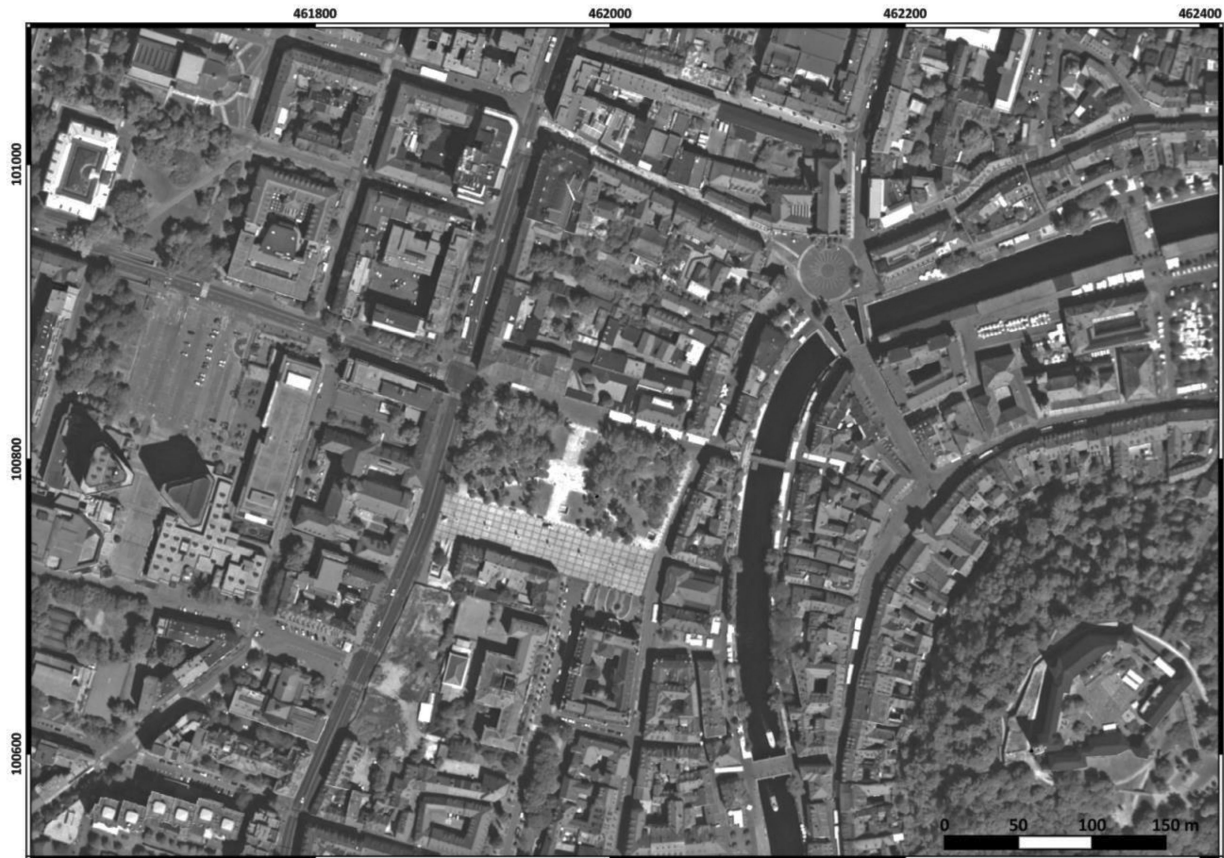
Fig. 16. Section of a true orthoimage.
