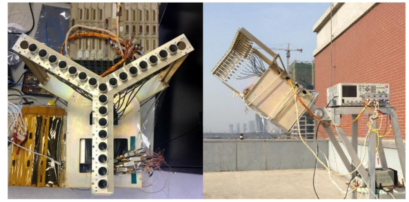
Fig. 6. Experimental equipment composition of X-band 2D synthetic aperture radiometer system.
