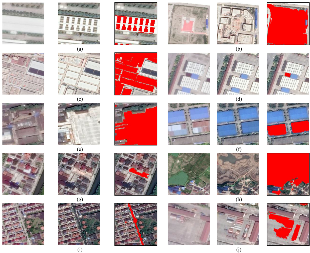
Fig. 24. Typical change types in Dataset 4. (a) Photovoltaic construction. (b), (c) Industrial park development. (d) Subtle change in industrial park. (e) Large residential area construction. (f) Roof repair. (g) Small residential demolition. (h) Park construction from farmland. (i) Road repair. (j) Temporary material stockpiles.
