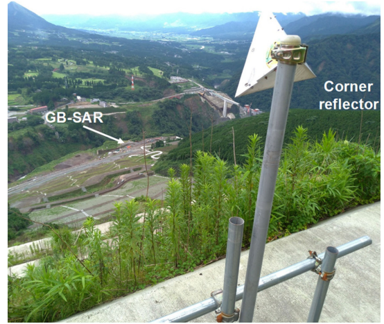
Fig. 8. One of the installed trihedral CRs at the observed slope.
