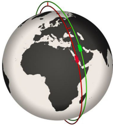
Fig. 2. Helix satellite formation. Red: TSX, Green: TDX; Typical baseline values vary from 120 to 500 m.
