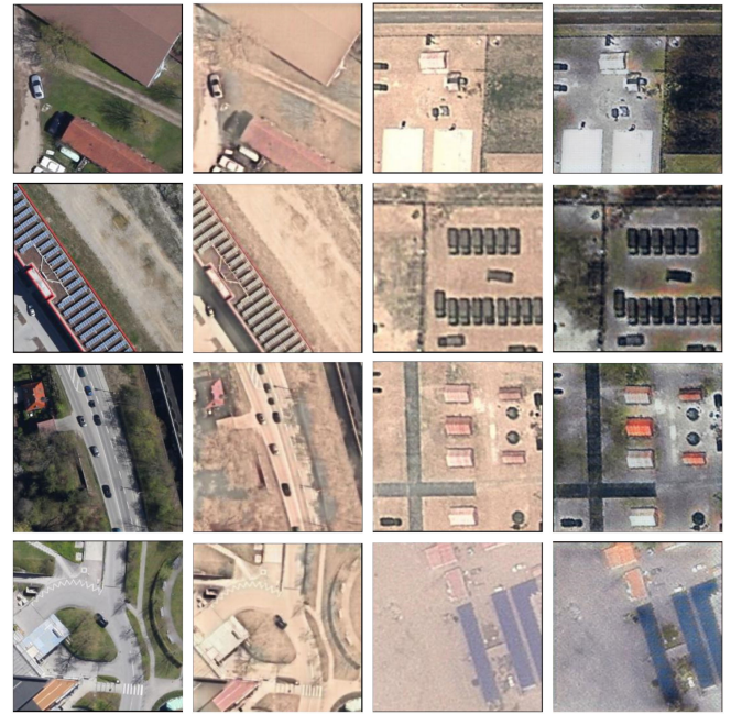
Fig. 1. Samples of the image enhancement using DE-CycleGAN. From the left column to the right column are DLR 3 K images, generated images from DLR 3 K images, weak satellite images, generated images from weak satellite images. The rightmost column is used for weak vehicle detection.
