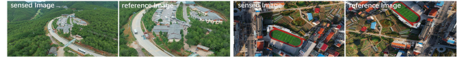
Fig. 8. Two image pairs used for training in our network, which contains in total 2072 SIFT putative matches (1349 inliers) as the training samples with 1349 positive samples and 1349 (including 626 misalignment samples) negative samples.
