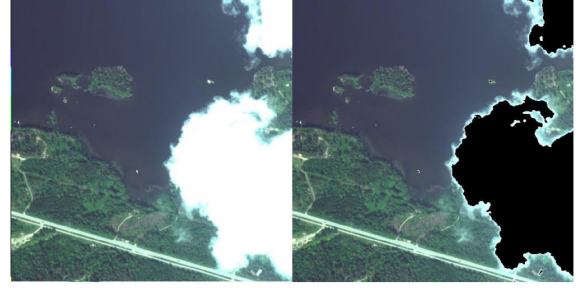
Fig. 7. Masked clouds from the WorldView-2 dataset. Left: Satellite image before cloud masking. Right: Satellite image after cloud masking.
