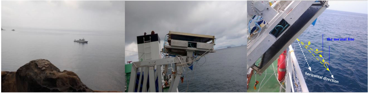
Fig. 9. Field campaign of the L -band array phased radiometer in the open ocean. (Left) The vessel in the experimental ocean area. (Middle) The radiometer pointing toward the sky. (Right) The L -band phased array radiometer pointing toward the sea surface.
