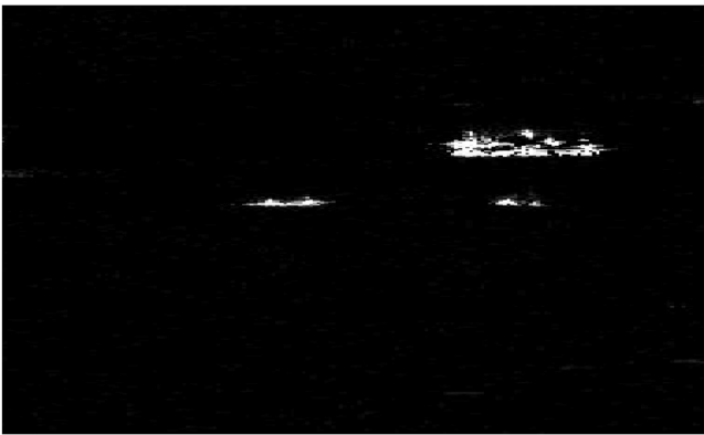
Fig. 12. Imaging results of multiple ships by measured single-channel SAR data.
