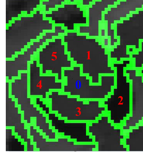
Fig. 2. Illustration of the spatially adjacent superpixels, where superpixels 1–5 are neighboring with superpixel 0. (Best viewed in color).
