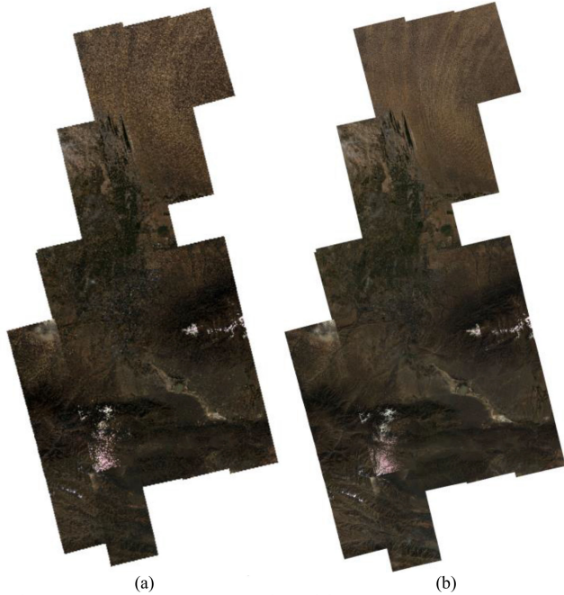
Fig. 14. Results of IRRA with or without global constraint. (a) IRRA without global constraint. (b) IRRA with global constraint.
