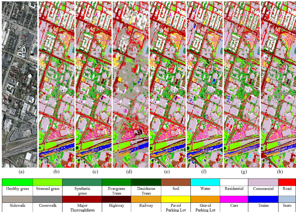
Fig. 14. Classification maps obtained by the different methods on the Houston University 2017 dataset. (a) RGB image. (b) Classification map obtained by the S-CNN method. (c) Classification map obtained by the CRVS-CNN method. (d) Classification map obtained by the MDR-CNN method. (e) Classification map obtained by the S-GAN method. (f) Classification map obtained by the W-GAN method. (g) Classification map obtained by the Self-GAN method. (h) Classification map obtained by the SA-GAN method (proposed).
