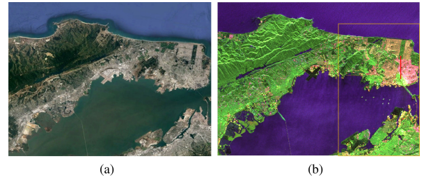
Fig. 2. Image of the study site in San Francisco, USA. (a) Optical image from Google Earth. (b) Corresponding color-coded Pauli decomposition obtained from the GF-3 dataset with red (double-bounce), green (volume scattering), and blue (surface scattering).
