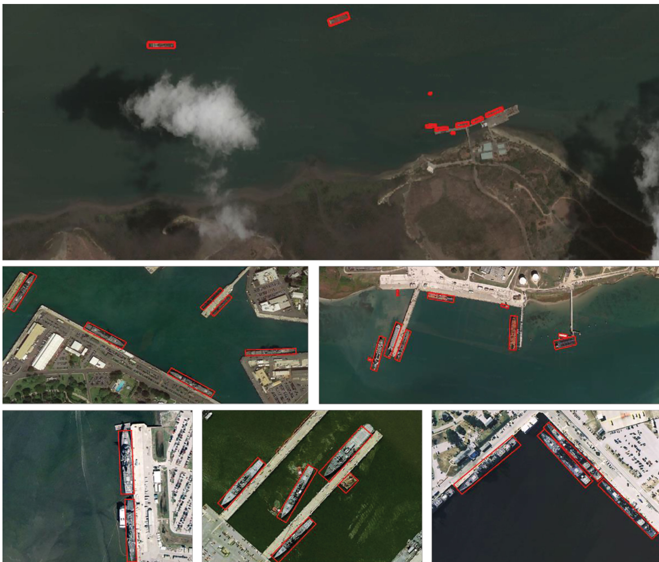
Fig. 11. Proposed inshore ship detection framework results from large view scale optical remote sensing images.
