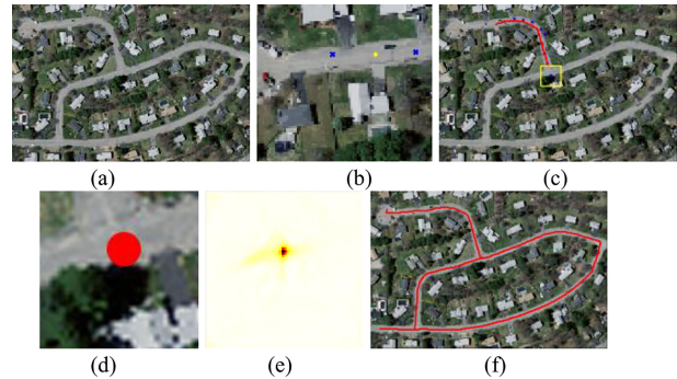
Fig. 6. Sliding window for road topology tracking. (a) Input image. (b) Seed is shown in yellow dot and the extension points estimated by the local spectrum analysis are shown in blue crosses. (c) Current step of the sliding window where the corresponding patch (yellow rectangle) is cropped to predict road central points. (d) Cropped patch and the predicted road central point. (e) Corresponding road center probability map inferred by our road center estimation network. (f) Final result.
