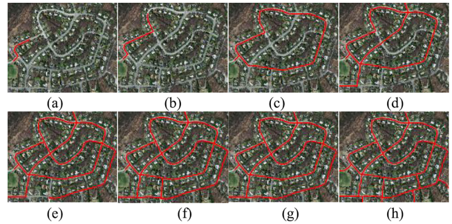
Fig. 12. Evolution of the road network by sliding window. The progress is displayed from left to right and from top to bottom.
