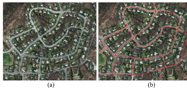
Fig. 2. Road network extraction from aerial images. (a) Input image. (b) Road extraction via our method.
