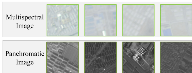
Fig. 1. Intra-class variations. Images of the same class (high building) captured by panchromatic and multispectral sources [5].
