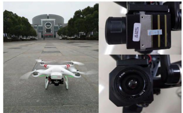
Fig. 3. UAV and thermal infrared camera.
