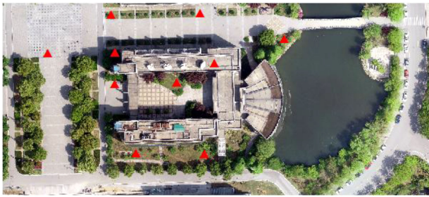
▲ The position of the temperature and humidity sensor
