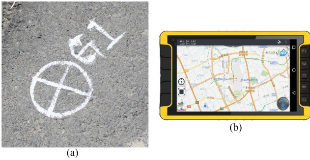
Fig. 2. (a) GCPs landmark. (b) Huace LT600T Client.
