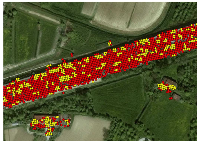
Fig. 7. High speed railway Padua–Venice, Italy. Very high density PSP analysis of COSMO-SkyMed Stripmap SAR data (50 ascending acquisitions, May 2009–September 2011). Many additional PSs (in red, or dark gray for black and white version of the paper) with respect to those found with standard processing (yellow points, or light gray) can be identified by intensive PSP processing. The measurement points are projected on a regular grid corresponding to the COSMO-SkyMed image posting, to highlight that they correspond to almost all the pixels of the SAR image in the areas where a coherent signal is expected.
