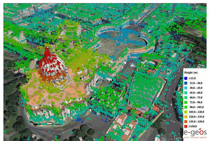
Fig. 4. St. Peter's Basilica, Rome, Italy. PSP height measurements obtained from COSMO-SkyMed Stripmap SAR data (34 ascending acquisitions, January 2010–May 2012). The 3-D view highlights the accurate positioning of the PSP measurements.
