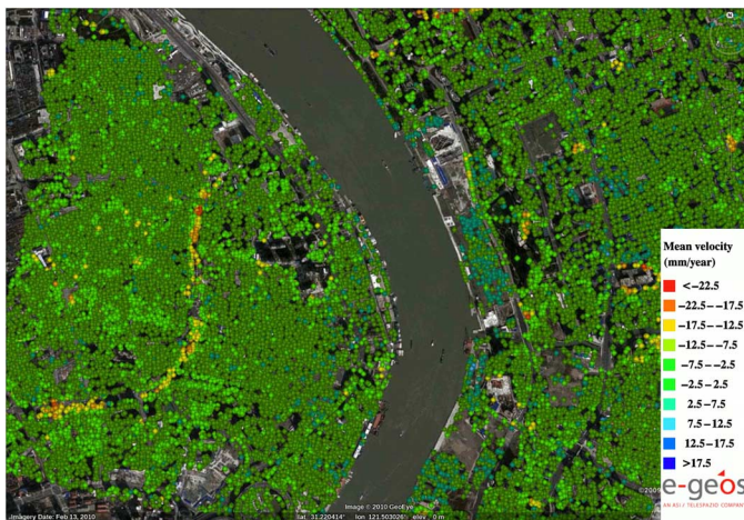
Fig. 6. Shanghai, China. Subsidence along the track of the subway line 9 detected by PSP mean velocity measurements from COSMO-SkyMed Stripmap SAR data (52 descending acquisitions, May 2008–June 2010).
