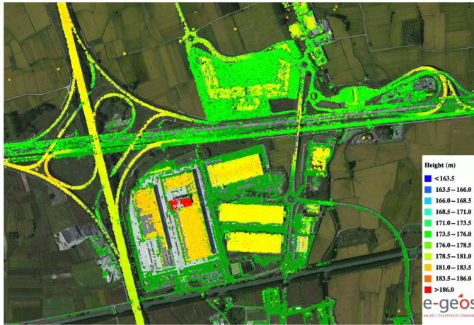
Fig. 9. Very high density PSP height measurements precisely reconstructing structures such as link roads, highway, railway, warehouses, etc., near Novara, Italy, obtained from COSMO-SkyMed Stripmap SAR data (30 ascending acquisitions, February 2011–June 2013).
